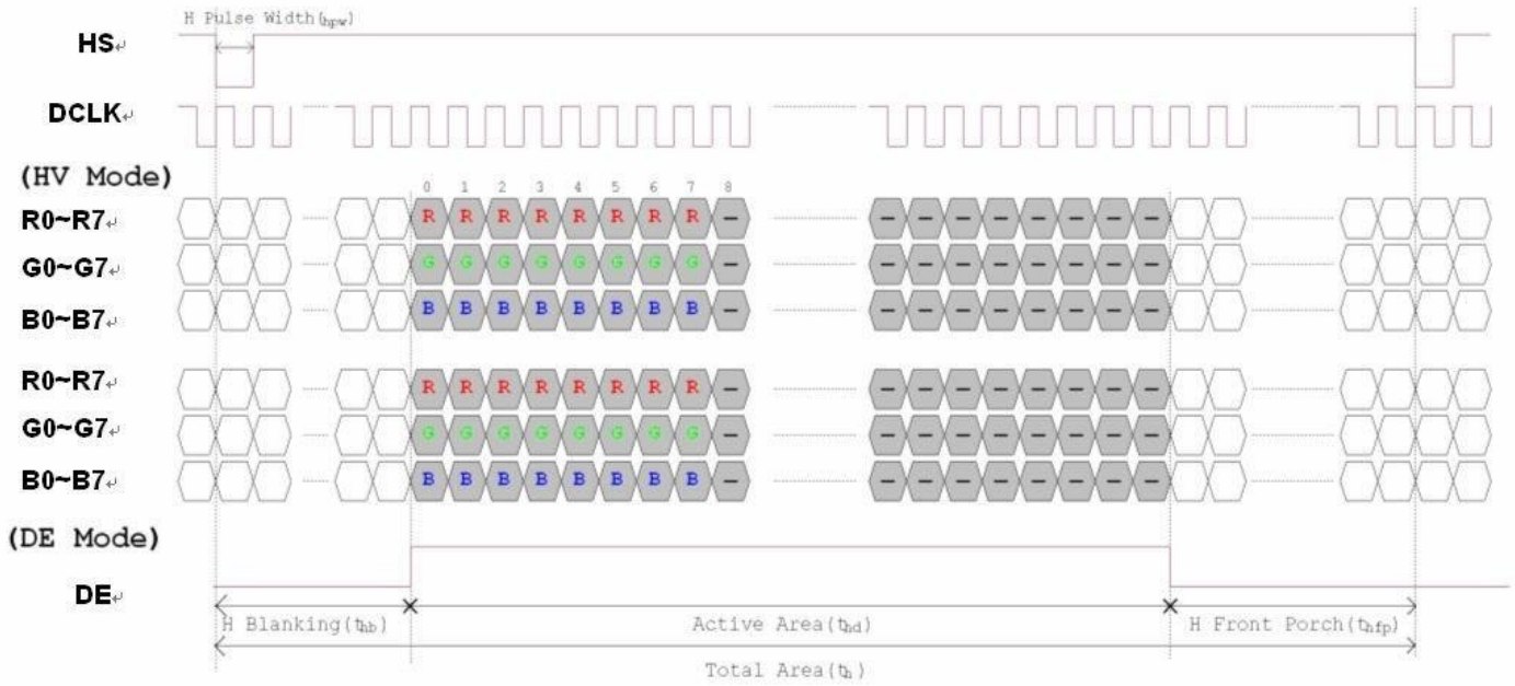
Figure 5.5.1 horizontal input timing diagram
