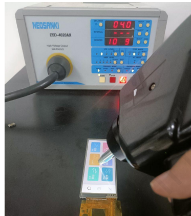
4.1 Electrostatic discharge test
