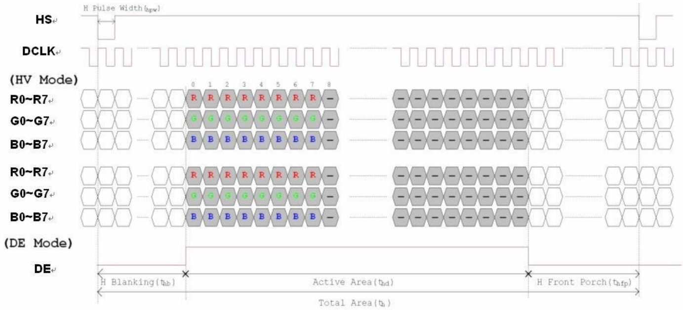
Figure 5.5.1 horizontal input timing diagram
